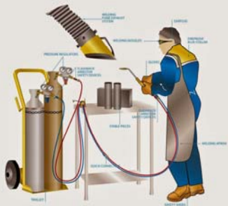
Correct and safe oxygas welding station
